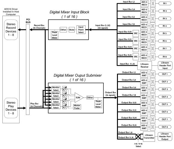
Figure 4: Signal Flow Diagram
