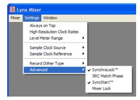
**SynchroLock™** – When checked, enables the SynchroLock clock generator. This should be disabled only when locking to external clocks that are near the limit of the SynchroLock lock range. Enabled by default.
