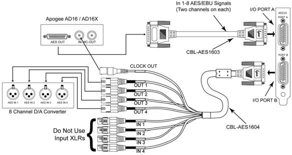
The AD16X is connected to the AES16 via our CBL-AES1603 cable, which is specifically designed to accommodate the Apogee 16-channel converters through their D-Sub port. I/O Port B in this example is connected to an 8-channel D/A converter using our CBL-AES1604 cable with standard XLR connections.
