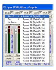
In this example, Digital In 1 is being selected as a monitor source for Output 1 Left. The "M" button next to the Output Monitor Source button must be in the "out" position to unmute a monitor source. After the source is selected, a corresponding four-letter pneumonic will appear on the button.
