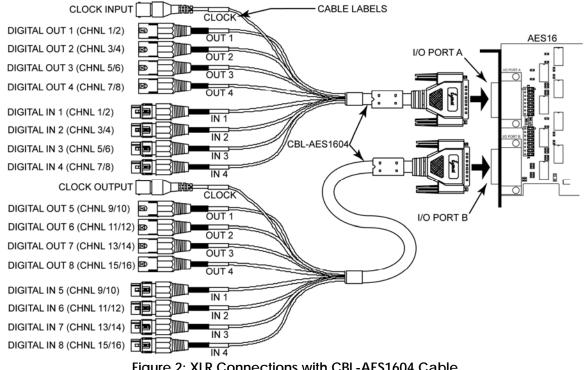
Figure 2: XLR Connections with CBL-AES1604 Cable
