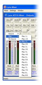
Selecting Play 2 (P2L and P2R) in the next set of Monitor Source Buttons down, and unmuting this source, allows you to monitor audio from Play 1 and Play 2 out of Digital Out 1 at the same time. If one application or playback stream is assigned to Play 1, and another to Play 2, you would hear audio from both out of Digital Out 1. You can adjust the relative level of these two sources with the volume slider directly underneath each Monitor Source Button.
