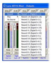
When a button is clicked, a pop-up menu is launched that displays the available sources that can be selected. A **Record** submenu lists inputs and their corresponding the record devices (which is dynamically updated to reflect Input Source selections in the Record/Play window). A **Play** submenu lists the left and right channels of the eight play devices. The **No Source** option disables a monitor source.
