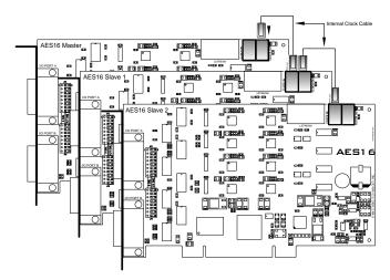
Figure 3: Synchronizing Multiple AES16's Using Internal Clock Connections
