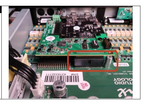
Screw the LSlot card into the standoff with the screw that was removed in step 3. Do not tighten.
