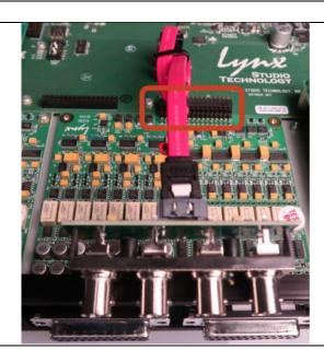
Insert the 2 included machine screws holding the LM-AIO8E to the mainboard. DO NOT TIGHTEN.
