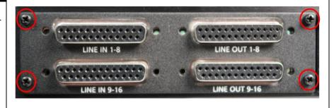
Screw in the D-Sub jack screws for the original I/O board. If installing an LM-AIO8E board, you'll need to screw in the D-Sub Jack screws that came with the new board. If installing an LM-A4 or LM-A24 monitor card, use the washers and nuts that came with it to secure the ½" jacks
