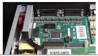
Insert the 2 included machine screws holding the LM-AIO8E, LM-DIG, or LM-A4/A24 to the mainboard. DO NOT TIGHTEN.
