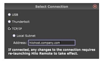
If the Host Computer is separated from the Target Computer/Tablet across a wide-area network (such as behind a router with NAT [Network Address Translation]), you will need to specify the router's IP Address and open port 5645 to forward to your Host Computer. Port 5646 is used to communicate between the Host Computer and the Target Computer/Tablet, so you would need to open port 5646 to forward to the Target Computer/Tablet.
