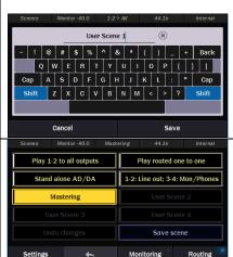
An onscreen keyboard will appear for inputting the scene name. Click the "x" at the end of name field to delete the factory name, if desired.
