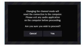
Clicking on the button will toggle Hilo between 16 channel (96 kHz maximum) and 8 channel (192 kHz) modes. You should not change this mode while an audio application is utilizing Hilo. This control resets the LT-USB and all audio will stop. When you press the button, you'll see this warning screen:
