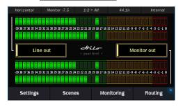
The horizontal meters are designed to show accurate level information with Peak Hold on two sources simultaneously. It can be helpful to keep an eye on a summed output while also viewing input signal strength.
