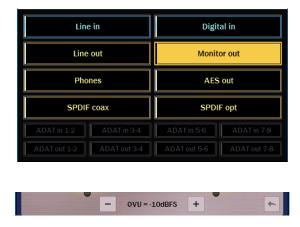
To select the meter source, press into the Source Select button below the Meters and select the desired source. Inactive sources will be grayed out.
