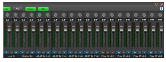
The purpose of this pane is to show input signal meter activity, allow assignment of physical inputs to record devices within the operating system, and manage the levels, routing, and pan positions of input signals being monitored through Hilo outputs.
