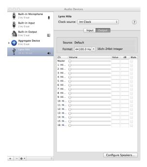
In cases where the playback software does not provide access to output selections, the default output devices for the operating system will be used. In OS X, the audio out default device can be established from Applications > Utilities > Audio MIDI Setup.
