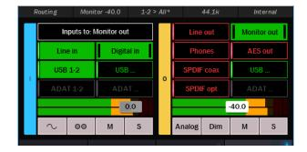
As you can see, the page is divided into input sources on the left and outputs on the right. What we are seeing here is which input sources are assigned to the displayed output. We are not turning inputs On and Off, we are turning the connection between an input and output On or Off. Think of it as a patch cables. Levels also can be managed here, both output levels and levels of monitor sources.
