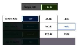
When Hilo is either clocked externally, or connected to the computer and subservient to the program or Operating System's rate (note: this is always the case with a USB connection to the computer), then the Sample Rate field is for display purposes only and is "grayed out".
