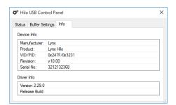
The third tab in the Hilo Control Panel opens the INFO page. This page simply reveals the connected product (again Hilo), the Revision of the LT-USB (its firmware version), serial number and driver build.
