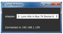
You should also see the "Connected to" indicator with the IP address of the Target Computer/Tablet show up on LynxRedirector on the Host Computer.
