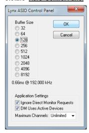
Many ASIO applications provide access to the driver's ASIO Control Panel. For a Hilo-TB, this button will launch the Lynx ASIO Control Panel.
