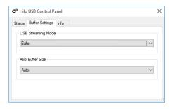
In the BUFFER SETTINGS page, the USB Streaming and ASIO buffer parameters control the size of the audio packets that are used to transfer audio to the LT-USB hardware. Smaller buffer sizes will give you lower latency.
