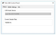
The STATUS page simply reveals the "USB Audio Device" (Lynx Hilo in this case), and the current "Sample Rate". The sample rate cannot be changed here, it is information display only.
