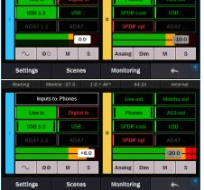
Now we'll add Line In, so the performer can hear their input signal. Again, we'll set the Monitoring Mode to "left" so their input signal is panned center in the headphones.
