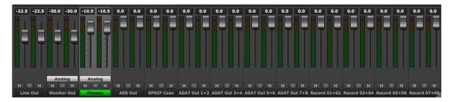
The Monitor Out and Phones channel strips have an additional button, just like in the Hilo's Routing page (see section 5.3.4: Routing). For these two outputs you can control both the digital output level and the analog output level. Clicking the button beneath the fader will toggle between Analog and Digital level controls.
