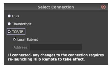
Simply uncheck the "Local Subnet" check-box, then enter the IP Address, Computer Name or Domain Name in the "Address:" field.
