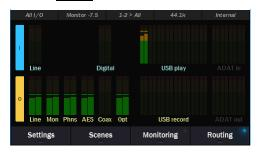
The All I/O meter page gives a global view of all input channels that are active and which outputs are receiving audio from at least one source. The ADAT I/O will be grayed out if the ADAT I/O is not active.
