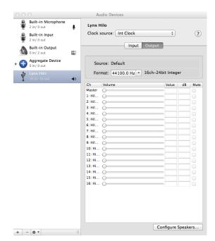
In cases where the playback software does not provide access to output selections, the default output devices for the operating system will be used. In OS X, the audio out default device can be established from Applications > Utilities > Audio MIDI Setup.
