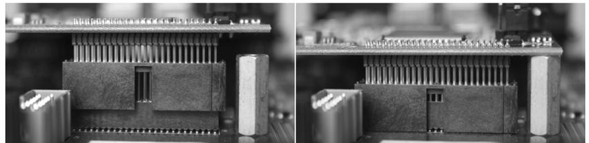
8. Secure the LT-DANTE with three screws; one into the standoff and two into the back panel of Aurora. Keep screws loose until the LT-DANTE is properly aligned, then tighten snugly, but do not over tighten.
