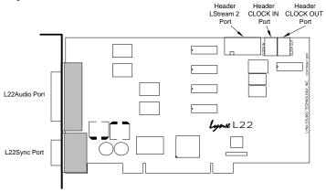
Referring to figure above, locate the L22Audio Port and the L22Sync Port on the mounting bracket of the Lynx L22. Insert the L22Audio cable into the L22Audio Port and tighten the thumb screws on the cable shell. Insert the L22Sync cable into the L22Sync Port and tighten the thumb screws on the cable shell.
