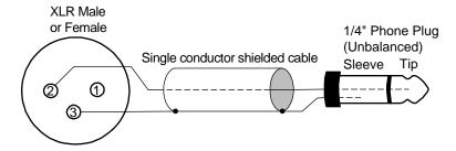
The wiring method for unbalanced connections with XLR connectors to unbalanced RCA/Phono phone connectors using coaxial cable (1 wire + shield) is as follows:
