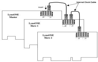
CLOCK OUT connectors on the MIDI/Clock Cable, use BNC cables to make connections between cards in the same sequence as described above.
