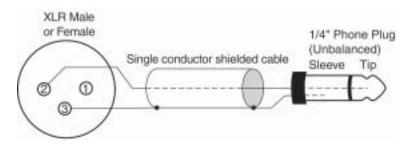
The wiring method for unbalanced connections with XLR connectors to unbalanced RCA/Phono phone connectors using coaxial cable (1 wire + shield) is as follows:
