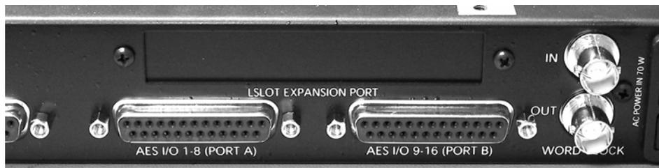
3. Mount the LStream LynxTWO Interface Bracket in the LSLOT Interface port. Secure with the two mounting screws which were removed in step 2.
