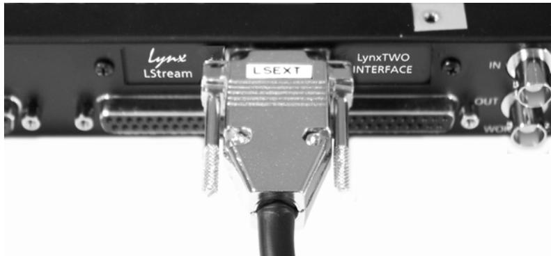
7. Connect the other end of the CBL-LSEXT to the sync port on the back of the LynxTWO/L22. Tighten thumbscrews until secure.
